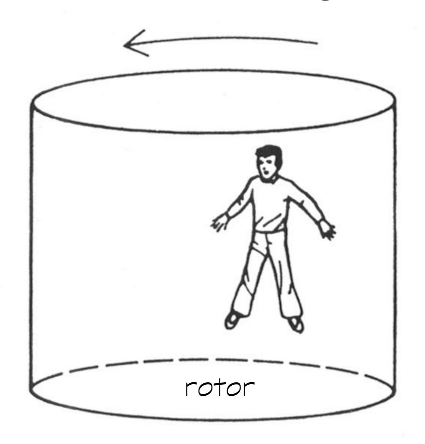
Once the inward centripetal force is broken the body will then move in a striaght line tangent to the circular path.
